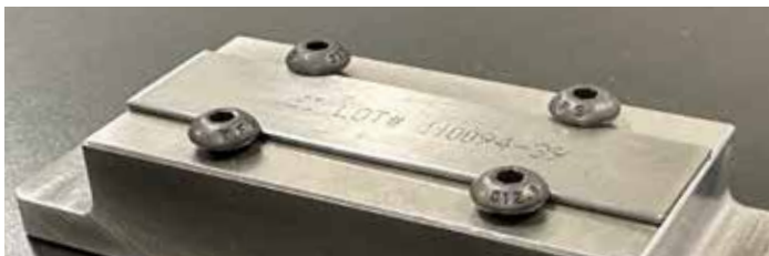
Almen A Strip fastened to peening test strip holder.
